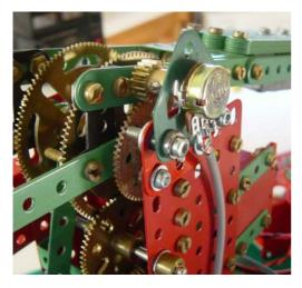
As the robot arm moves through its full range (about 80 degrees), the potentiometer is geared to move through most of its full 270 degree range and so provides a varying analogue voltage signal between 0 Volts at one end of the range (Analog value = 0) and 5 Volts (Analog value = 255) at the other end of the range.
