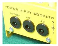
NOTE: THESE CONNECTORS MUST BE WIRED CORRECTLY – THE GROUND GOES TO THE PIN IN THE MIDDLE.
