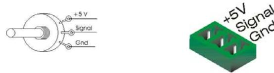
The simplest way to use these ports is with a Potentiometer. When wired as shown above, turning the knob on the potentiometer (which is just like the volume knob on a radio) will change voltage on the Signal line between 0 and 5 Volts.
